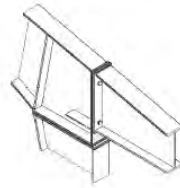
Built up Canopy
